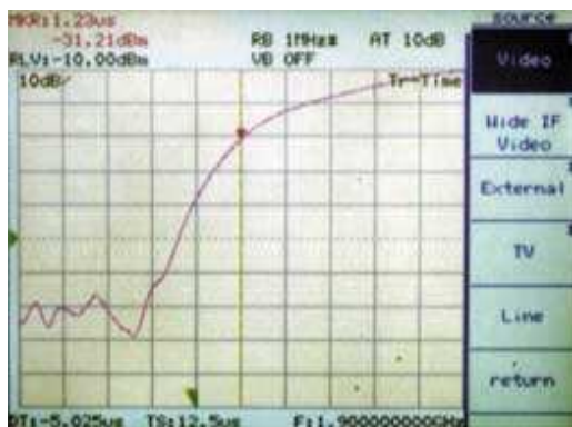
High-speed time-domain measurement (TS=12.5 \mu s)
